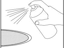
the paint with paint thinner will lessen the risk of filling any holes. If a hole gets plugged use a can of compressed air to open it. Once the paint is dry, put the cloth back on the grille.
